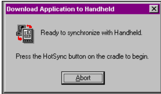
Figure 14. Press the Sync button your handheld cradle when ready to deploy your application and tables from the SatForms IDE to your handheld.
