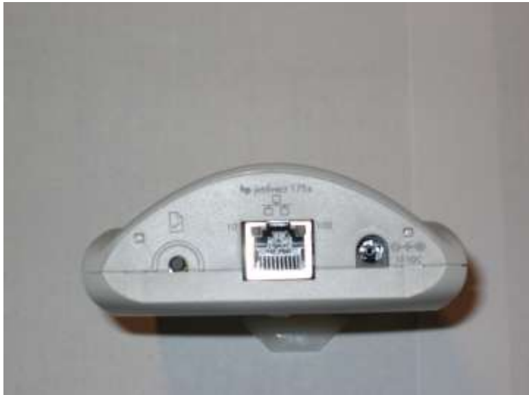
Figure 3. The back of the Hewlett-Packard JetDirect has two connections and a button.
