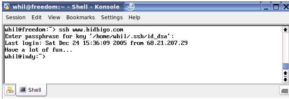
Figure 9. After SSHing into a remote box, you'll be prompted for your passphrase.
