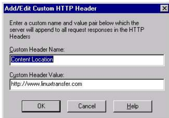
Figure 7. Use the Add/Edit Custom HTTP Header dialog to define headers for a virtual host.
