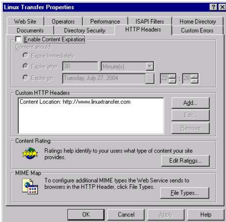
Figure 6. The HTTP Headers tab allows you to define custom headers for virtual Web sites.
